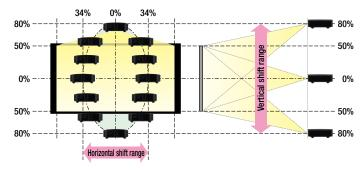
The vertical and horizontal lens shift function cannot be set to the maximum values simultaneously.
